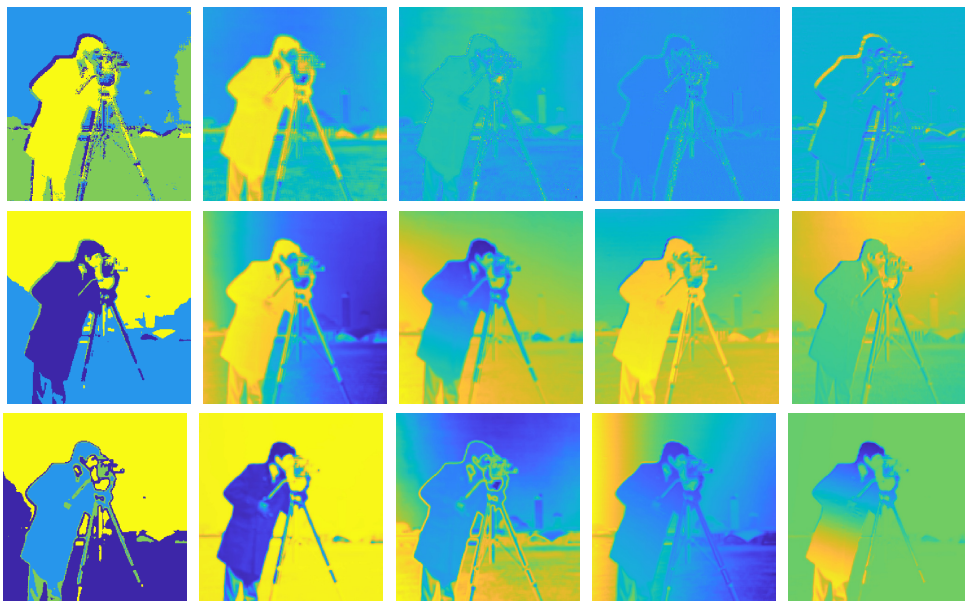
Figure 6: Clean cameraman. Top row, LLL: first image is the image segmentation result using top 4 eigenvectors, the second to the fifth images are top 1 to 4 eigenvectors. Second row is from Nyström and the last row is from Roseland.
