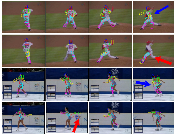
Figure 12: Examples of kinematic tracking on the baseball and figure skating data sets. The 1st and 3rd rows are our results. The 2nd and 4th rows are results of Ramanan (2006). Notice how mistakes of our method (blue arrows) still look like valid human poses, while those of Ramanan (2006) (red arrows) can be wild.
